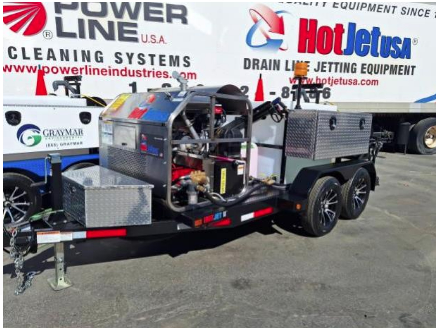
ECWC's hydraulic jetting/scrubbing unit
